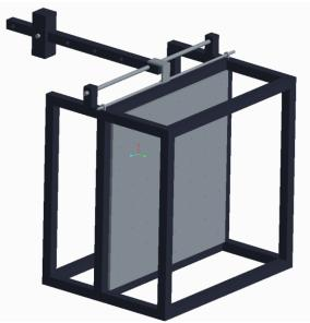
Fig. 4 - CAD solid model of our kinetic hammer apparatus
