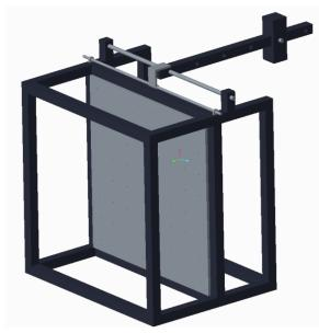
Fig. 5 - Final design in CAD utilizing a swing hammer
